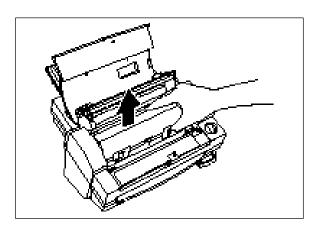
(4) Remove the film cartridge from the machine.
